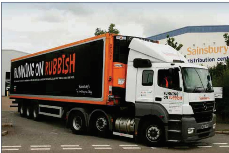
Trying something different: Mercedes-Benz Axor tractor retro-fitted with Clean Air Power's Genesis dual-fuel (diesel/LNG) system.
